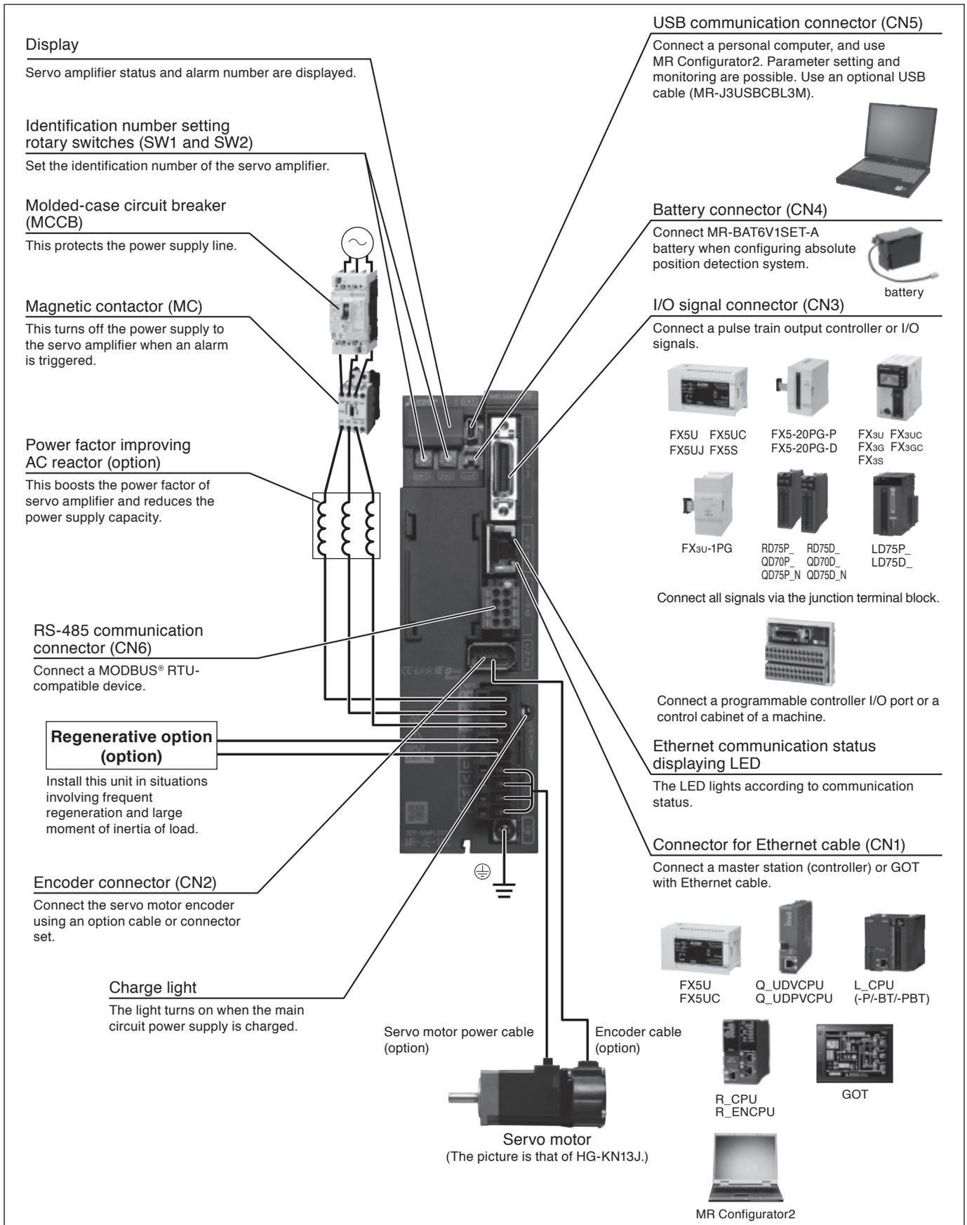
Notes: 1. The connection with the peripheral equipment is an example for MR-JE-100C or smaller servo amplifiers. Refer to "MR-JE\_C Servo Amplifier Instruction Manual" for the actual connections.
