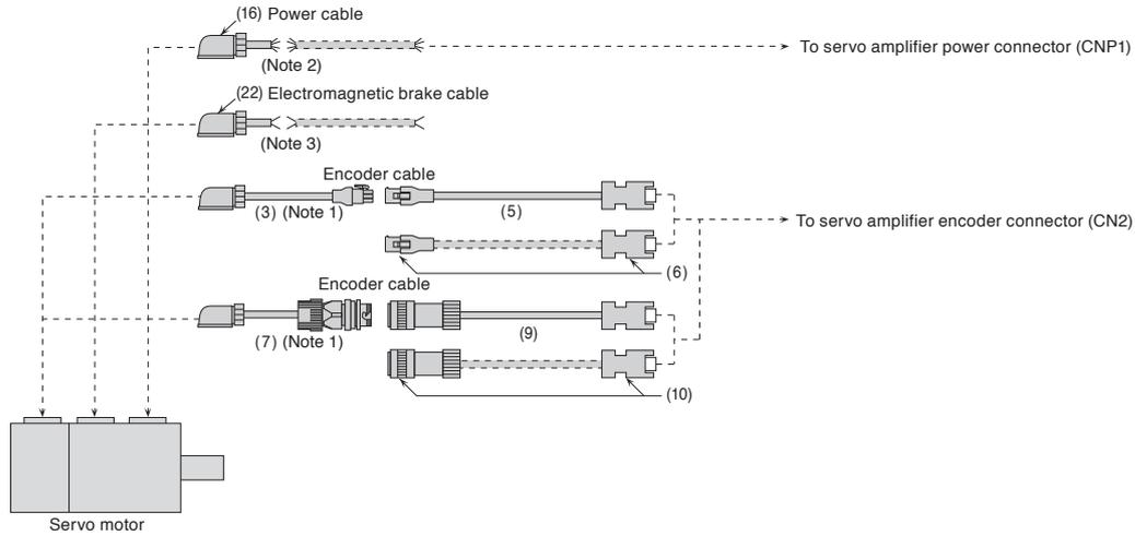
● For leading the cables out in the opposite direction of the load side (Note 4)
