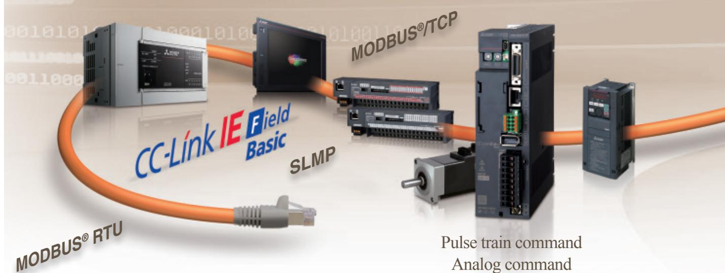
MR-JE-C servo amplifiers support pulse train command and Field Network. With a single servo amplifier, you can select a suitable interface from a variety of selections to configure a system.
