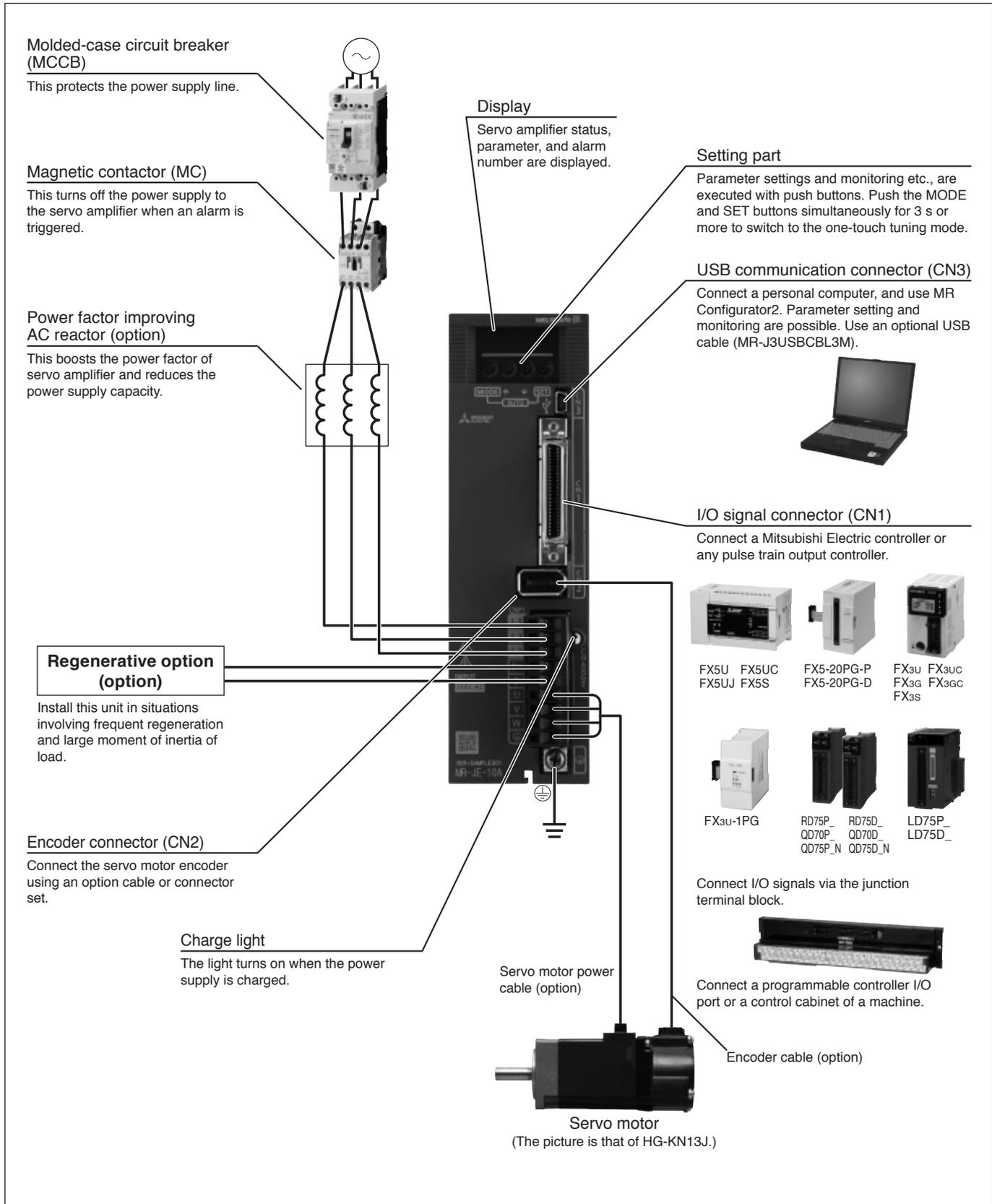
Notes: 1. The connection with the peripheral equipment is an example for MR-JE-100A or smaller servo amplifiers. Refer to "MR-JE-\_A Servo Amplifier Instruction Manual" for the actual connections.
