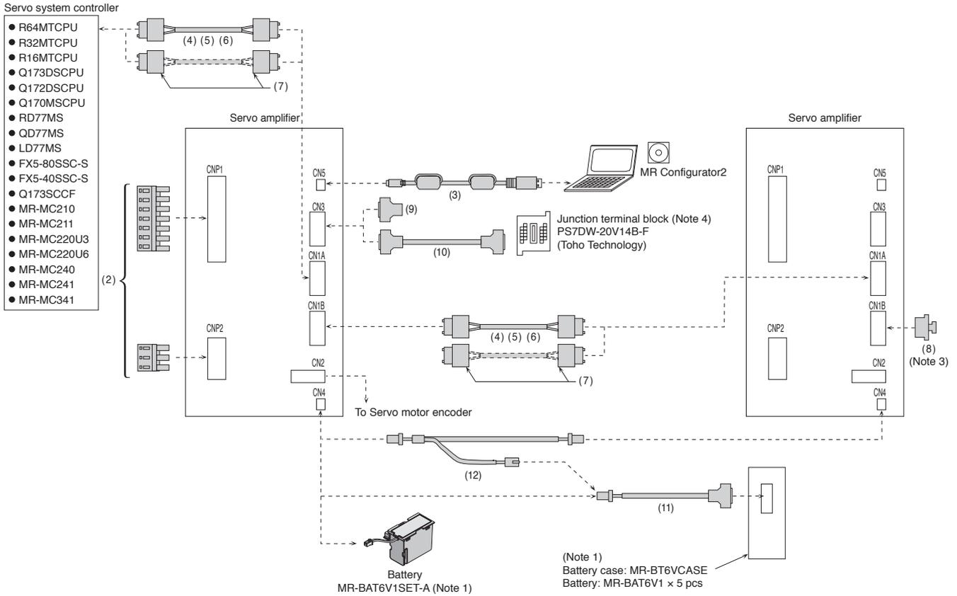
Notes: 1. Refer to "Battery" or "Battery Case and Battery" in this catalog. Battery and battery case are not required when the MR-JE-B servo amplifier is used in incremental system.
