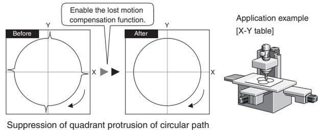
Suppression of quadrant protrusion of circular path
