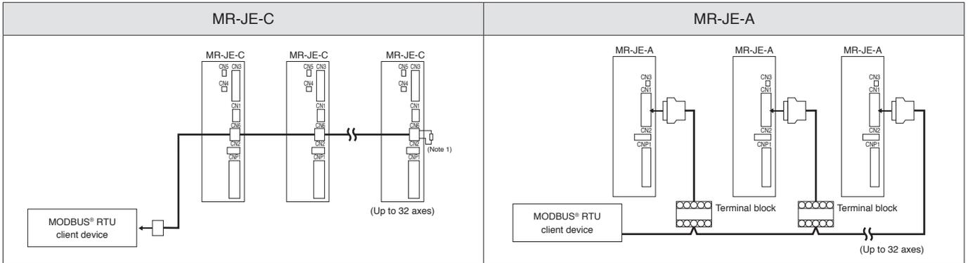
Notes: 1. For the final axis, terminate with 150 Ω resistor between DA and DB.
